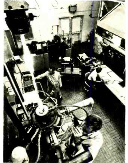
PILOT PRODUCTION LINE for making optical waveguides, now operating in Atlanta, GA. To make the lightguides, high-silica-content glass rods are prepared on a glass lathe (glowing area, upper right), then softened (upper left) and pulled into hair-thin fiber lightguides through equipment in lower left.
